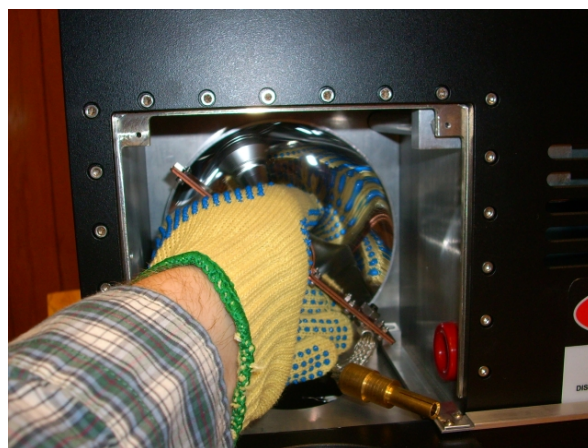
Figures 10 and 11 – Inserting the bulb assembly into the lamp chamber
