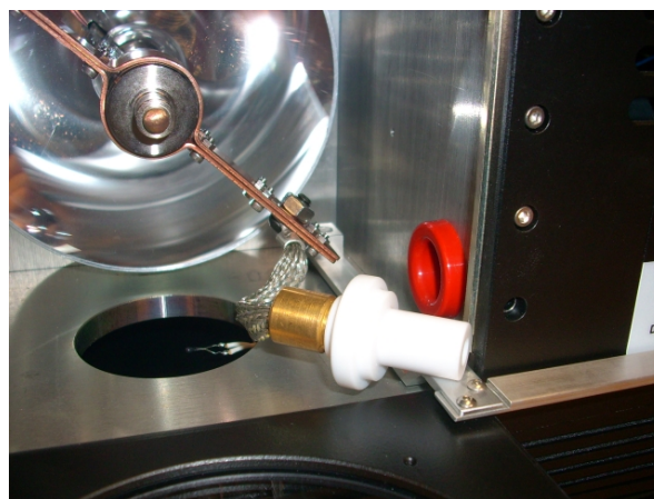
Figures 12 and 13 – Installing the Teflon insulator on the end of the anode connector
