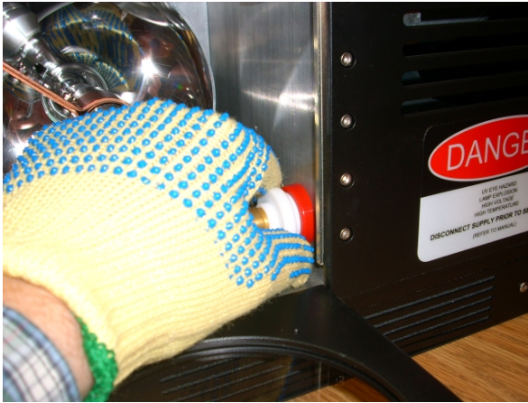
Figures 24 - 25 – Removing the anode connector from the side panel receptacle
