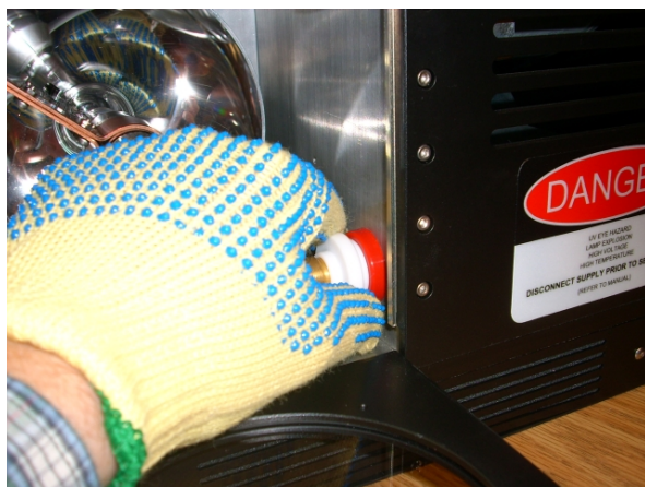
Figure 14 – Inserting the anode connector into the side panel
