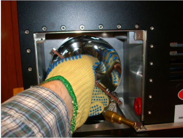
Figures 27 – 28 – Removing the bulb assembly from the lamp chamber
