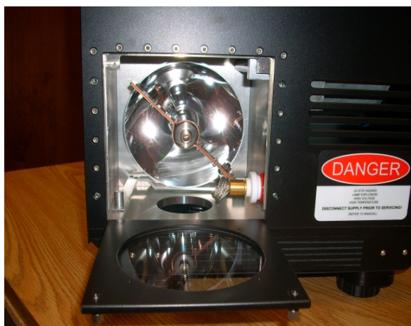
Figure 17 – Bulb in place, anode connector in receptacle, and bulb release lever closed
