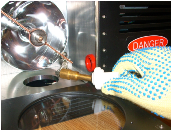
Figure 26 – Removing the Teflon insulator from end of the anode connector
