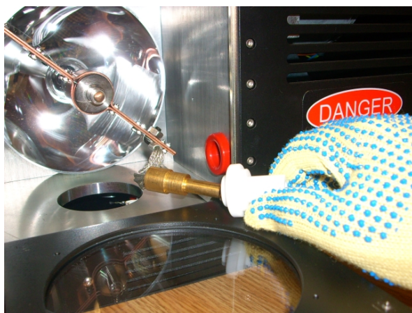
Figures 12 and 13 – Installing the Teflon insulator on the end of the anode connector
