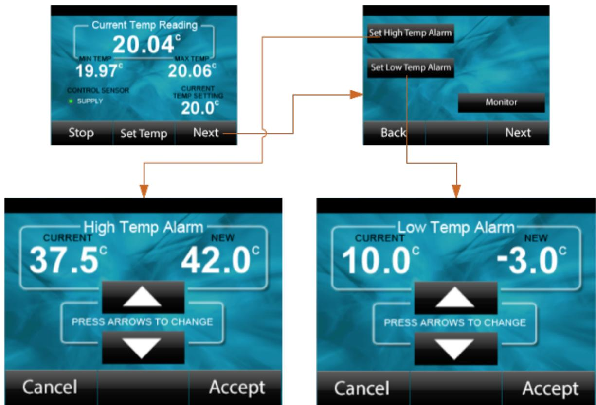
Figure 5-4: User Set Temperature Alarm Limits Screen
