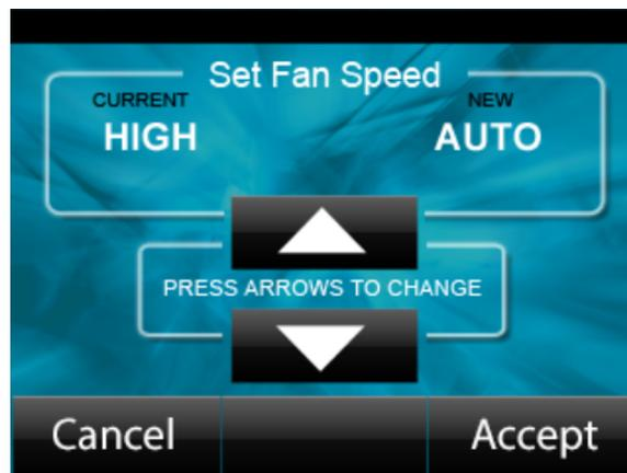
Figure 6-4: Fan Speed Selection Screen
